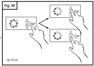
The more LEDs that are illuminated, the higher the force limit. For example, level 1 (least amount of force) is set when only LED #1 is illuminated. Level 2 is set when LED #1 and #2 are illuminated. Level 4 is set when LEDs #1, #2, #3, and #4 are illuminated. By repeatedly pressing the "+" or "-" button, the force can be increased (+) or decreased (-).
