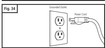
To reduce the risk of electric shock, your opener is provided with an insulated power cord with a 3-prong grounding plug. The cord must be connected to a standard grounding outlet. If there is no outlet available at the location, you must have a qualified electrician install an approved grounded outlet in this area.
